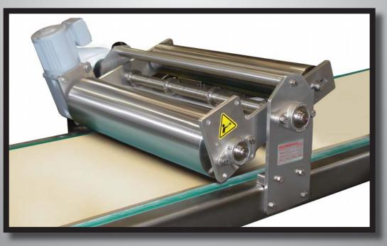
Powered Compression Roller with Gearmotor-Driven Roller
