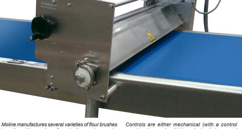
Moline manufactures several varieties of flour brushes to suit a wide number of production environments. These machines are designed to remove excess flour from the top of the dough sheet using a set of rotating brushes. The excess flour is removed either by auger or by vacuum for reuse.
