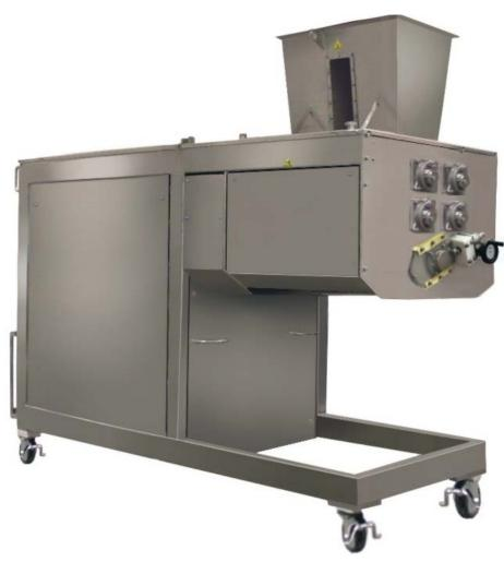
The LIBRA Quinto extruder provides low stress processing of very thick, high moisture doughs. The extruder contains five rollers. This combination provides consistent, low stress processing without overworking the dough, leaving cell structure open and loose. The extruder is manufactured in several sizes to produce dough sheets from 16" to 32" wide, at 2" thick or more. Typical production rate is 20,000 pounds per hour depending upon the application.
