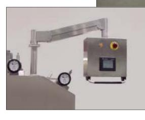
Level II: Operator interface mounted in articulating panel.
