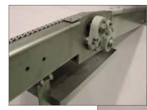
Standard Level I features: Stand-off mounting, outboard bearings.
