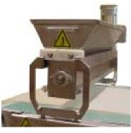
**Standard Flour Duster** Mounts directly to conveyor. Hopper slides out for flour removal and sanitation.
