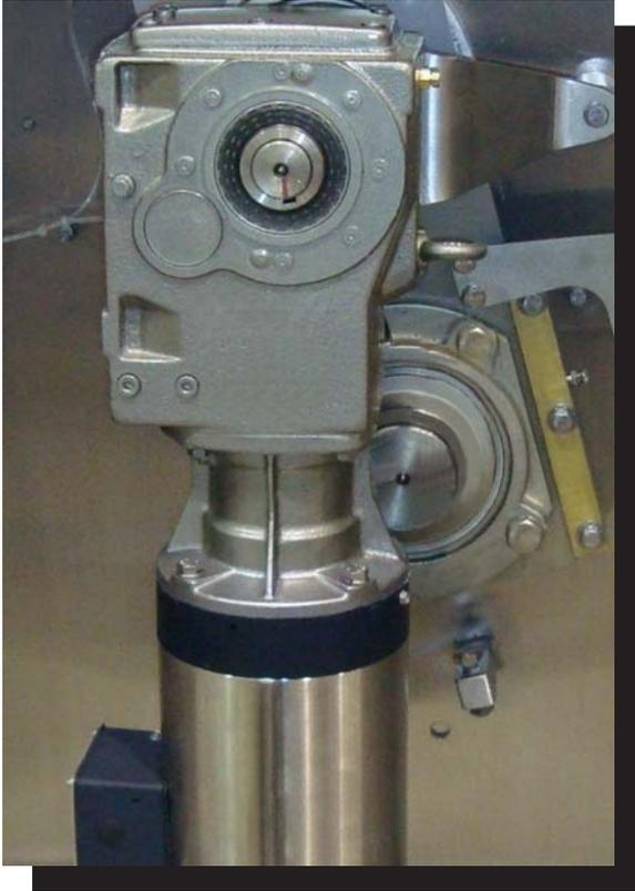
*Oversized Gearbox Drives and Piloted Bearings*
