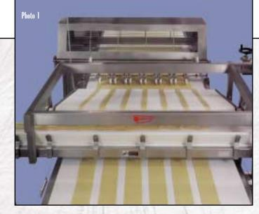
station for closed loop production (see Drawing 2). Options available on trim conveyors include smooth urethane belts, open surface plastic link belts that are positive tracking and cleated belts for inclines.
