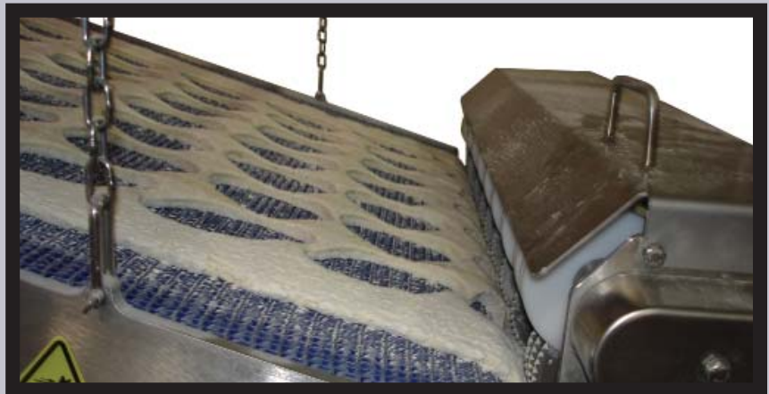
Reverse Trim Pickup Unit With Self Threader
