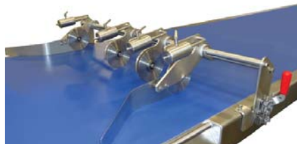
Counterweighted Strip Cutter and Trim Diverter Blades
