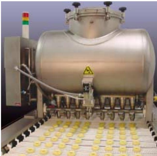
A Moline pressure cut donut tank at work.
