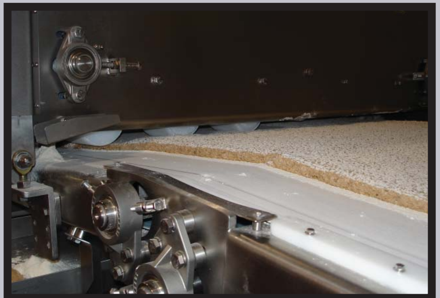
Cross Sheeting the Dough to Specific Width and Thickness
