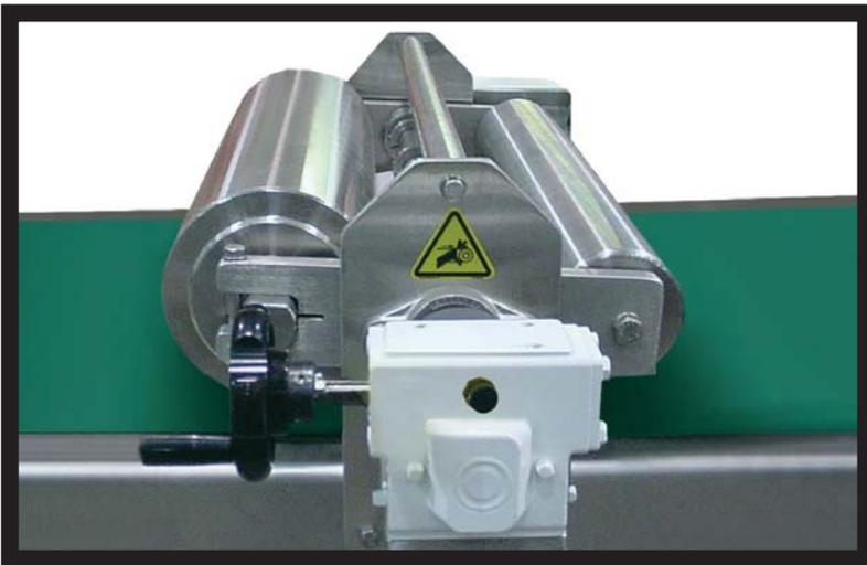
*Powered Compression Roller (with "motorized pulley")*
