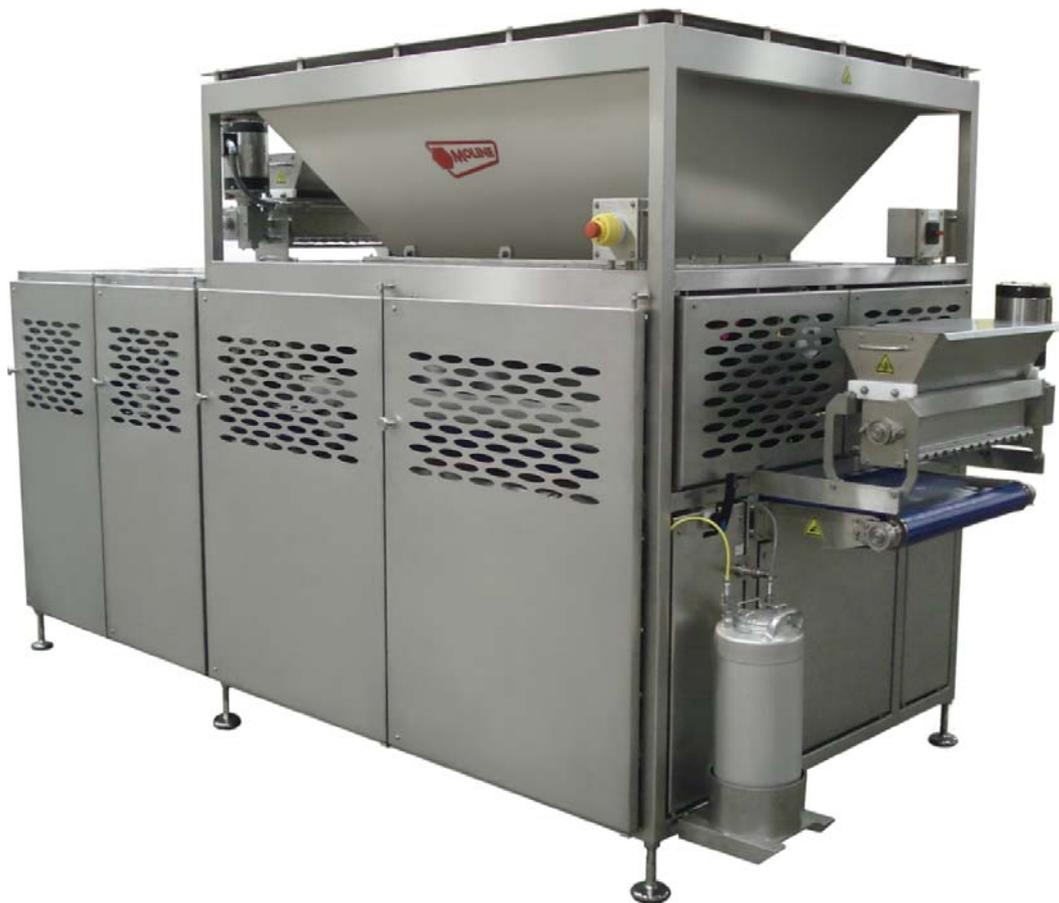
*The Moline YOGA dough sheet former is designed to deliver a true, stressless dough sheet for high-volume industrial applications. The unique three-stage design, incorporating portioning, multi-rolling and tamping/weight control, is perfect for variety bread systems, frozen or pre-fried donut systems, pizza, pita and flour tortilla lines. The unit consists of a chunker with hopper and starwheel portioning paddles, a satellite roller, tamping roller and conveyors.*
