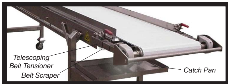
Telescoping Belt Tension Mechanism, Belt Scraper and Catch Pan
