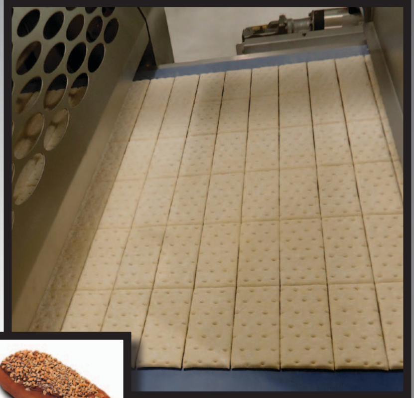
Stamping Die for Long Johns in Operation
