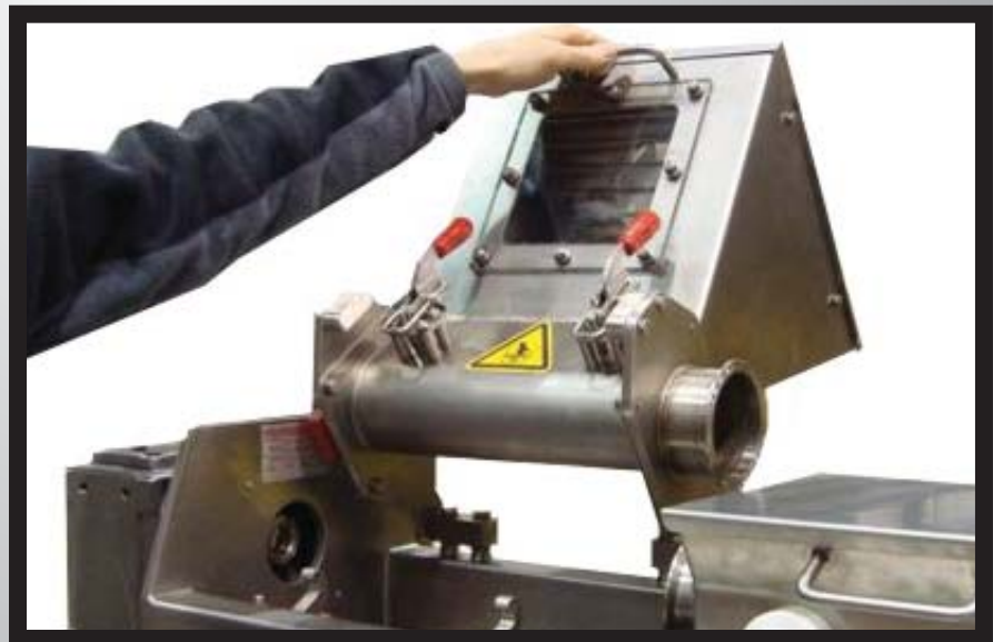
Rotating the Intake Hopper
