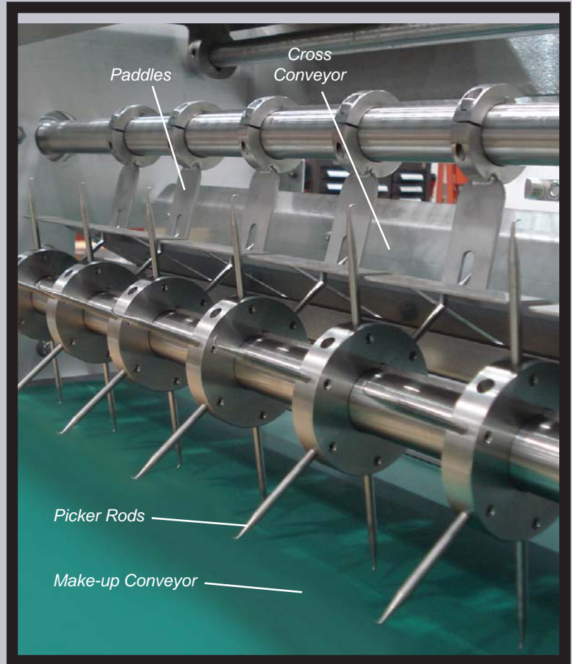
Portable Donut Hole Removal Unit (interior) (shown with guard open during shutdown)
