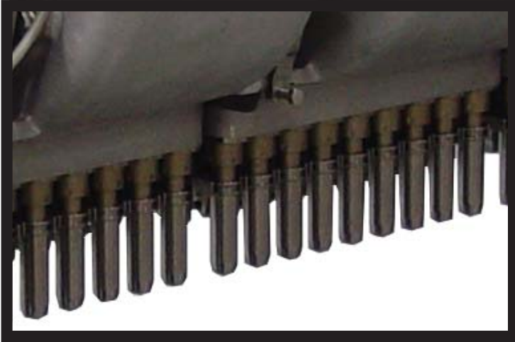
Cake Donut Cutters Mounted in the Depositor
