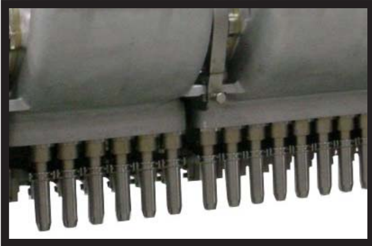
Cake Donut Cutters Mounted in the Depositor
