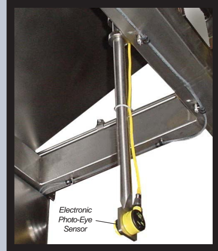
Dough Sensors on Chunker Frame
