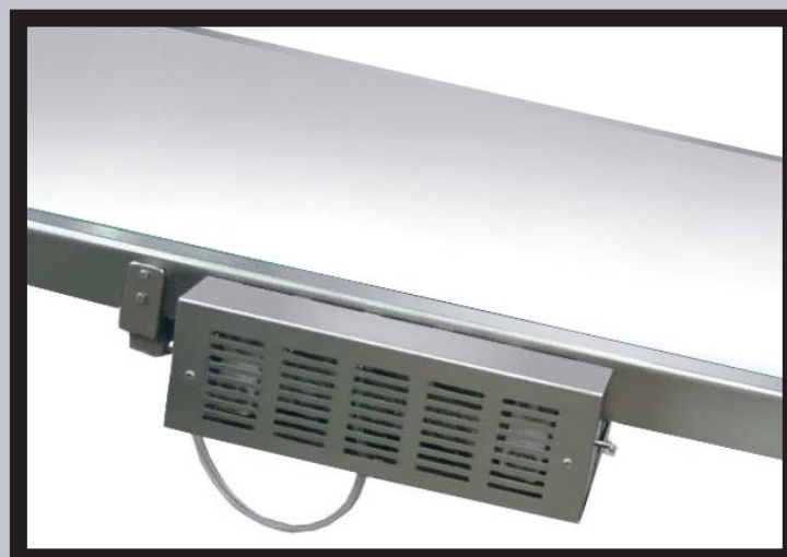
Belt Tracker With Front Guard Installed
